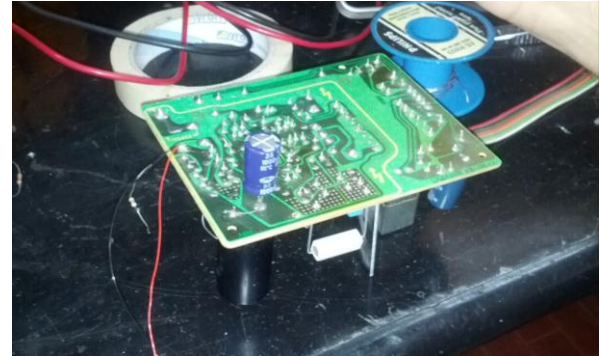
Fig. 10. Rectifier used for the test
