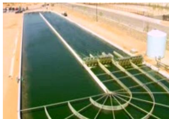
Fig. 1, Algae growing in an open raceway pond 3
