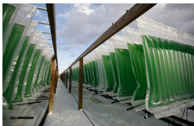
Fig. 2, Algenol facility produces ethanol in a closed bag system 5
