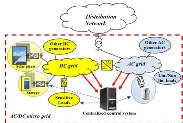
Fig. 1, The hybrid AC/DC  $\mu$ G general scheme.
