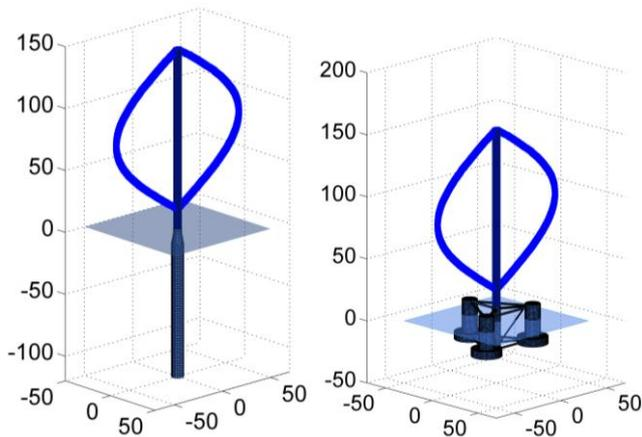
Fig.1: Left – spar-type floating VAWT; Right – Semi-submersible floating VAWT.
