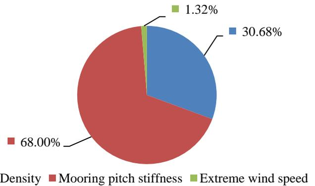
Fig. 2: Importance factors of the stochastic variables in estimation of the reliability index for the spar-type floating VAWT.
