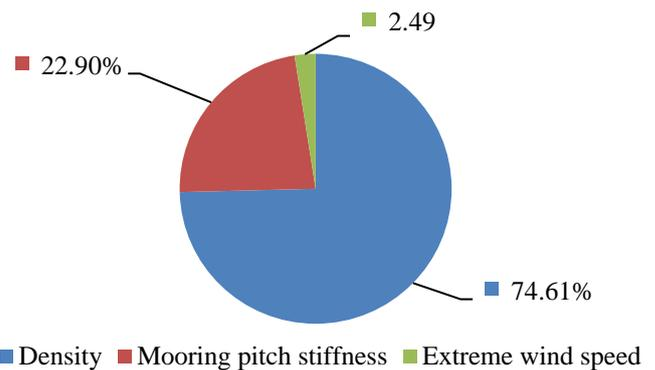
Fig. 3: Importance factors of the stochastic variables in estimation of the reliability index for the semi-submersible floating VAWT.
