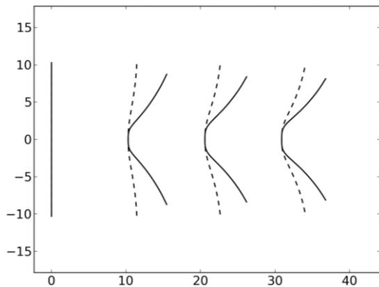
Fig.13, Multi-stage HF driven by fluid pressure  $p_{hf}=q^{s-1}$ ,  $q=1.2$ ;  $T_1=0.65$  and  $T_2=0.8$  ( $k=1.23$ ) and  $d/2a=0.5$ .
