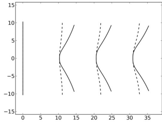
Fig.10, Multi-stage HF driven by fluid pressure  $p_{hf}=q^{s-1}$ ,  $q=1.4$ ;  $T_1=0.4$ ,  $T_2=0.8$  and  $d/2a=0.5$ .
