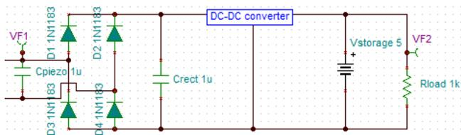
Fig. 5. Scheme of the energy harvesting circuit.
